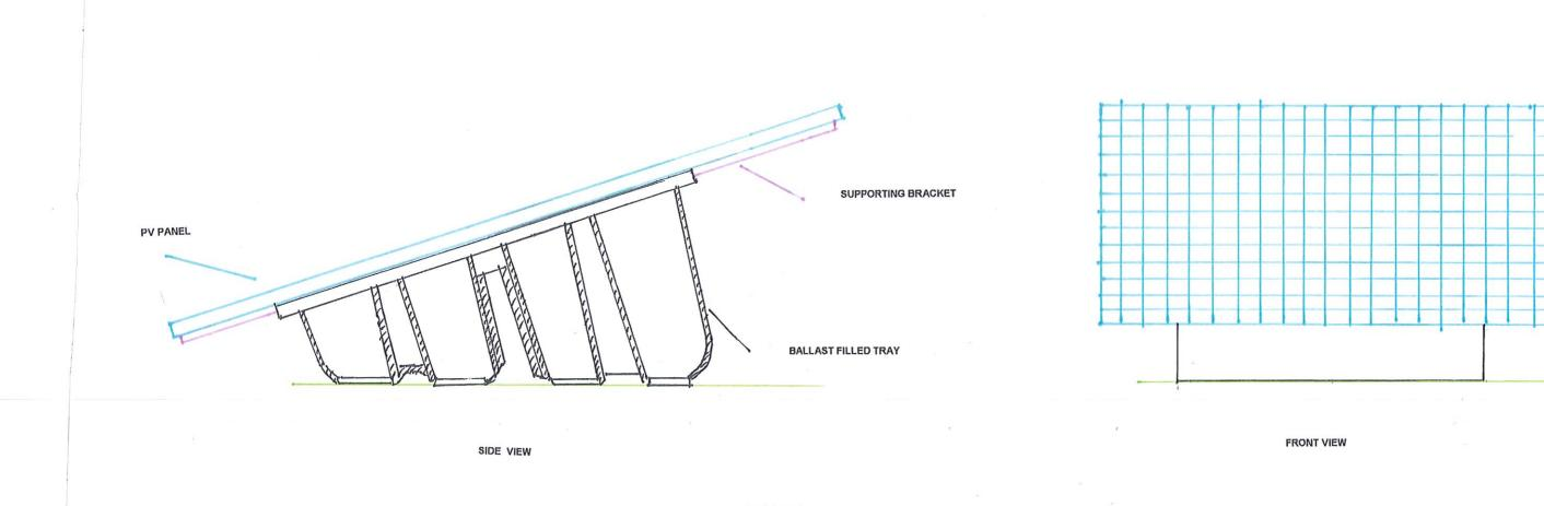
Two adjacent solar arrays are proposed as shown on the submitted site block plan. Each array unit will consist of one Fastensol Tray (as specified in the accompanying data sheet) filled with gravel, supporting one solar PV panel (see separate data sheet).
